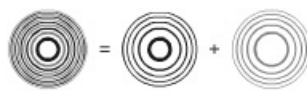
Figure 2 | An illustration of the overlay nanofabrication technique for micro zone plate fabrication. The zone plate is composed of even-numbered opaque zones (black and grey) and odd-numbered transparent zones (white). Set I (black), containing zones 2, 6, 10, ... and its complement, set II (grey), are fabricated sequentially to form the desired overlaid micro zone plate.
