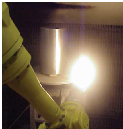
A robotic arm holds the plasma torch for manufacturing ceramic nanocoatings.
