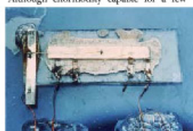
Then: the first integrated circuit (above), invented by Jack Kilby (right), and now: Intel's Pentium 4 microprocessor (top right).
